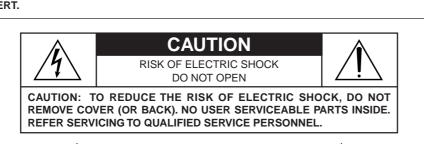
The lightning flash with the arrowhead symbol within an equilateral triangle, is intended to alert the user to the presence of uninsulated "dangerous voltage" within the product's enclosure that may be of sufficient magnitude
